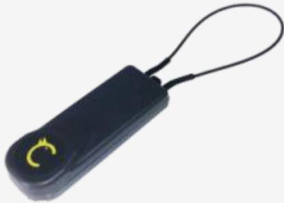
If a tag is taken too far away from the Hub, the alarm will sound until it is returned to the zone or deactivated with the Remote. The Tag is also jam-proof - if you try and conceal or block the signal between the Tag and Hub then the alarm will also sound.
